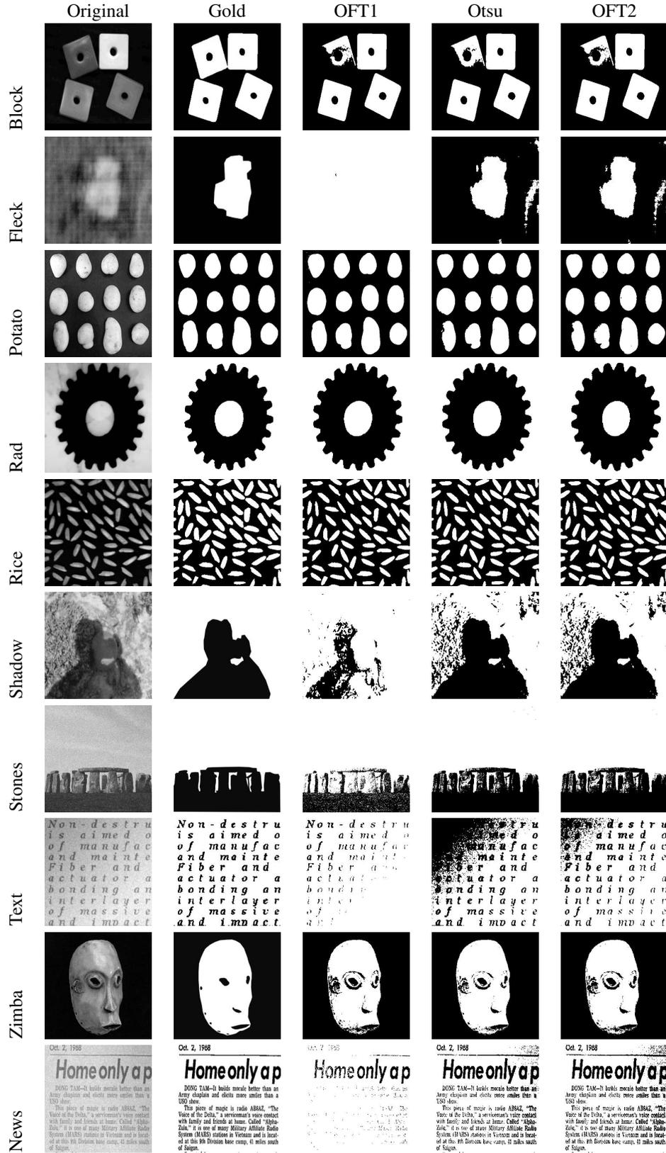
Figure 5. Test set of general images and corresponding results for the three algorithms, OFT1, Otsu method, and OFT2 (proposed).
