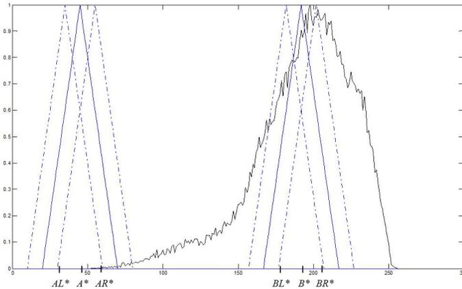
Figure 3. Proposed oppositional fuzzy set image thresholding algorithm, the six different sets ( $A, AR, AL, B, BR, BL$ ), with their centers ( $A^*, AR^*, AL^*, B^*, BR^*, BL^*$ ) are illustrated. The distance between  $A^*$  and  $AR^*$  is  $\Delta$ , analogously for  $A^*$  and  $AL^*$ ,  $B^*$  and  $BR^*$ ,  $B^*$  and  $BL^*$ . The width of all fuzzy sets is  $2\delta$ .
