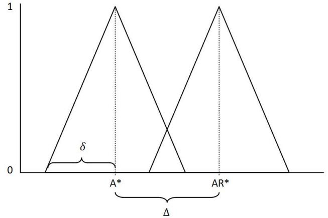
Figure 4. Illustration of  $\Delta$  and  $\delta$ .  $\Delta$  is the distance between the centers of the original set and created sets to the right and left.  $\delta$  is half the width of the fuzzy set.
